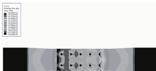
图2 复合材料多钉连接结构应力分布 Fig.2 Stress distribution of multi-fastener joints composite laminates
